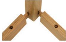
Interlocking corner block and rail joint lends superior strength at critical joints and provides optimum support for the seat suspension. This provides more durability and comfort for the life of the chair. All chair frames are reinforced with screws, not just glue, for rigidity and durability. Solid wood corner blocks provide support at all critical joints.
